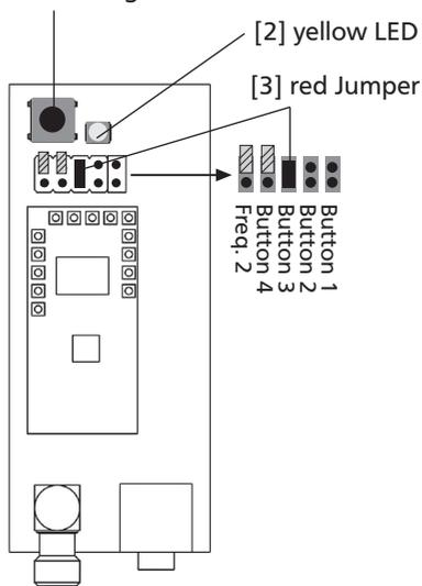
Fig. 2: Button 3 activated, Jumpers on Button 4 and Freq. 2 inactive (stored).
