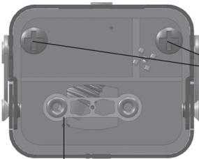
6: · Screws for connecting the vaporizer to the connecting pins
